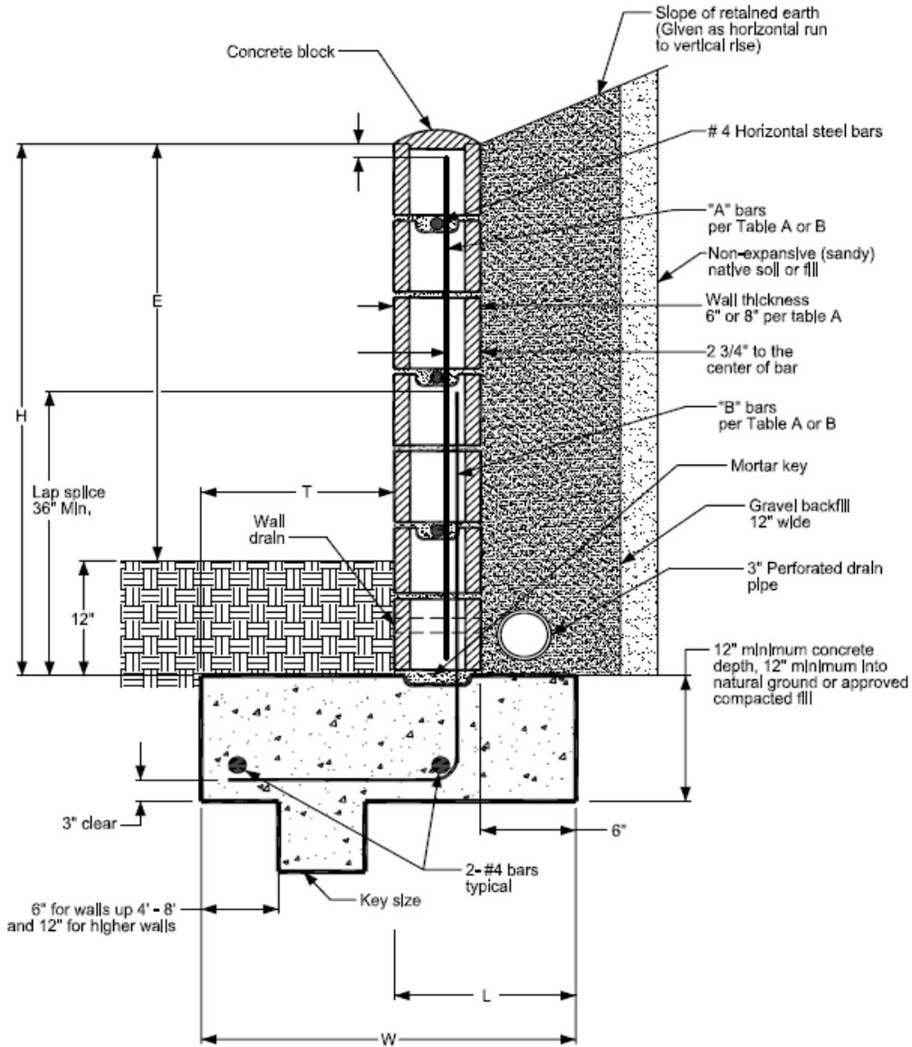
Figure 4 / Type III Retaining Wall with Level Sloping Backfill
