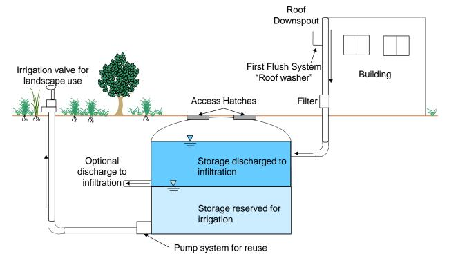
FIGURE 5-6. Schematic of a Typical Cistern
