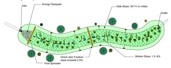
FIGURE 5-10. Schematic of a Vegetated Swale
