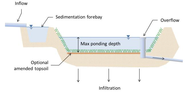
FIGURE 5-7. Schematic of a Typical Infiltration Basin
