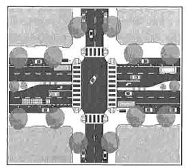
A curb ramp is a short ramp cutting through a curb or built to it. It provides an accessible route that people with disabilities can use to safely transition from a roadway to a curbed side walk and vice versa. It is difficult or even impossible for a person using a wheelchair, stroller, walker, or other mobility device to cross the street if the sidewalk does not provide a curb ramp. If curb
