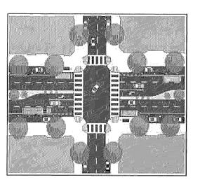
A curb ramp is a short ramp cutting through a curb or built to it. It provides an accessible route that people with disabilities can use to safely transition from a roadway to a curbed side walk and vice versa. It is difficult or even impossible for a person using a wheelchair, stroller, walker, or other mobility device to cross the street if the sidewalk does not provide a curb ramp. If curb
