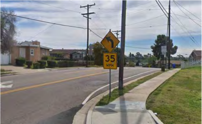
2 ADVANCED CURVE WARNING SIGN
