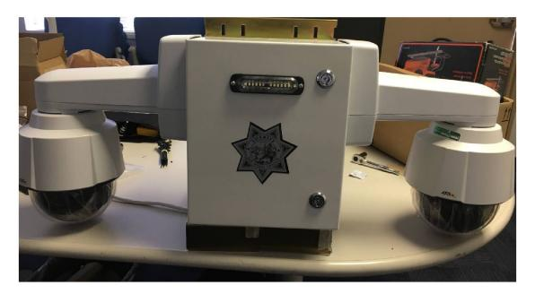
The installation of the cameras will be completed by a Sheriff's Contractor who is skilled and possesses the necessary certifications to mount these to existing light poles. The only necessity for these cameras is power which can be obtained from the light poles that have already been identified for use.
