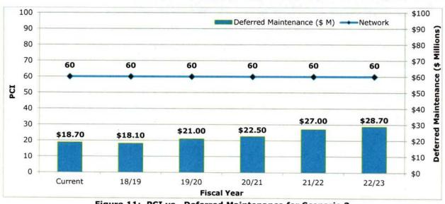
Figure 11: PCI vs. Deferred Maintenance for Scenario 3
