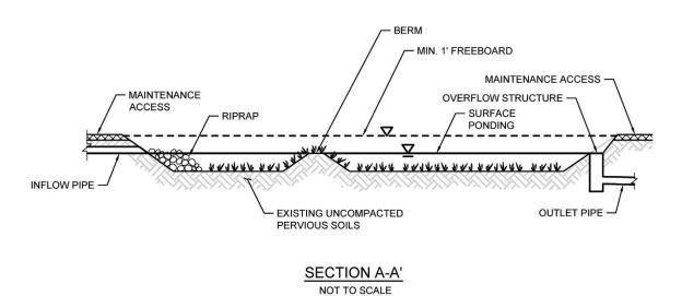
Typical plan and section view of an Infiltration BMP
