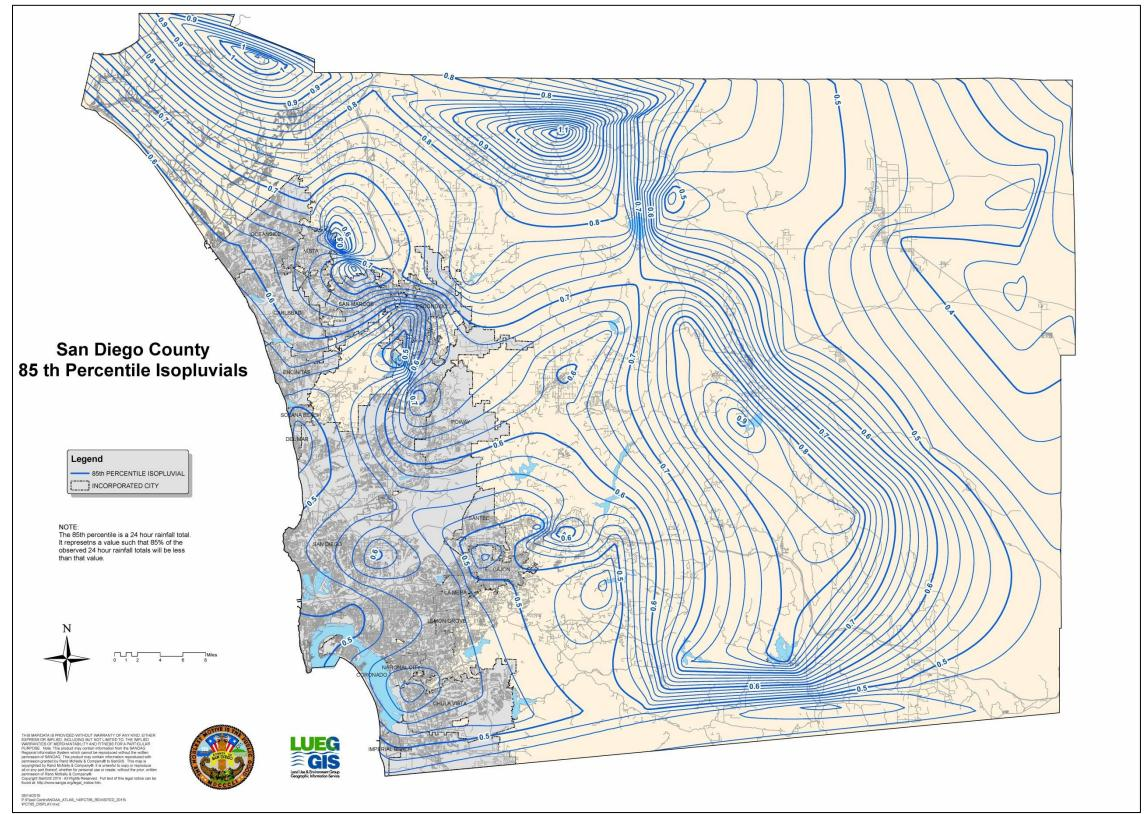
Figure B.1-1: 85th Percentile 24-hour Isopluvial Map
