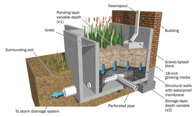
Biofiltration with impermeable liner BMP Example Illustration
