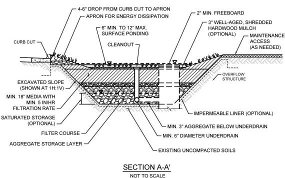
Typical plan and Section view of a Biofiltration BMP
