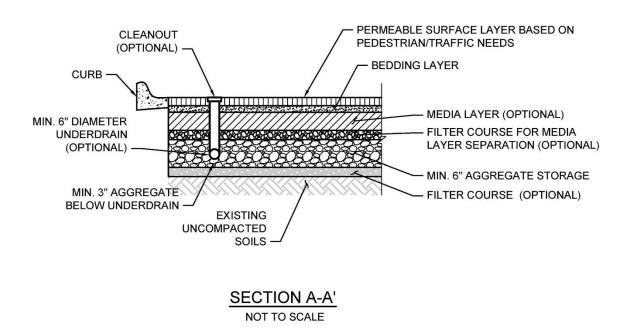
Typical plan and Section view of a Permeable Pavement BMP
