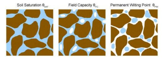
Figure G.1-4: Soil saturation, field capacity, and wilting point
